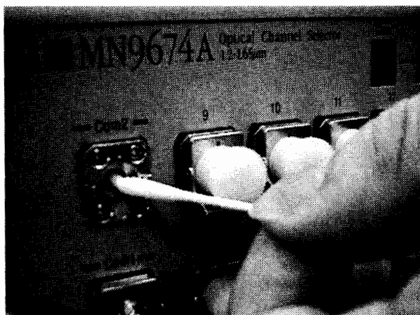
Figure 7-2 Cleaning using cotton swabs
