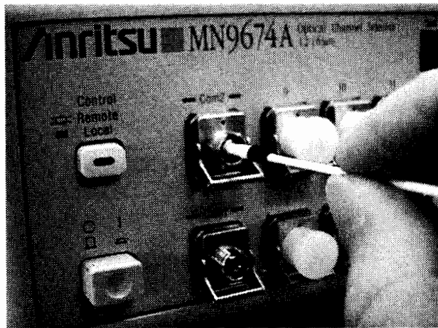
Figure 7-1 Cleaning using an adapter cleaner
